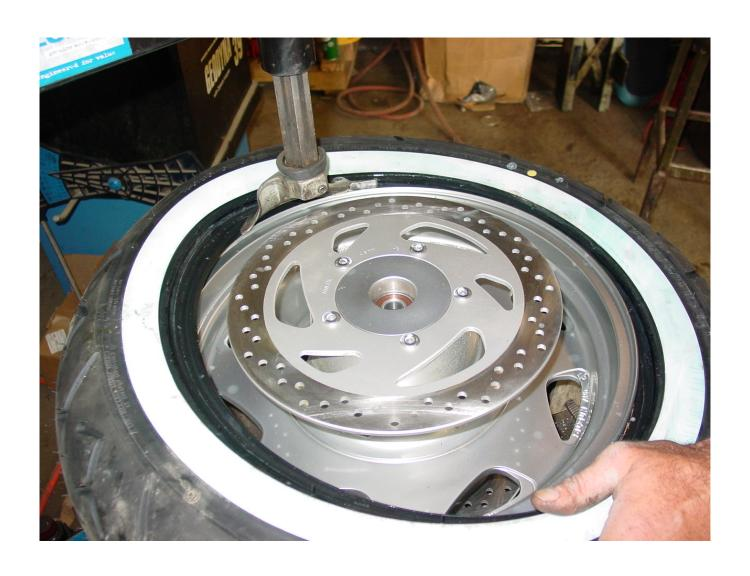
Carefully work the second tire bead down over the rim.
