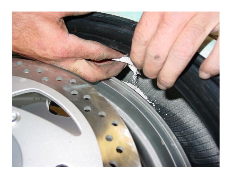
Carefully pour the beads into the concave portion of the tire.
